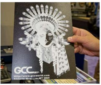
Fig. 2: GCC's white inks can be used as an undercoat, a spot color or as an overprint. Here you're seeing a white graphic printed on black media.
